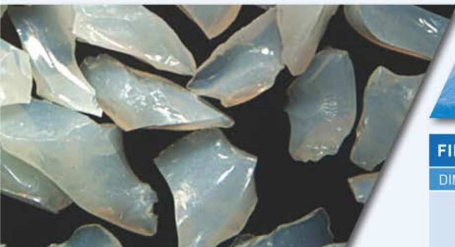
SG new generation - sharper edges generate an aggressive and low energy cut
